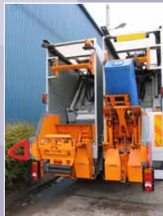
The automatic reverse raise function brings the binlift chairs to a high level, this action minimises the possibility of equipment damage whilst performing reverse manoeuvres.
