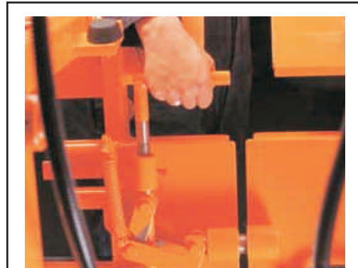
One simple operation of the manual chair lock ensures both lifting chairs are locked securely together for trade collection duties.
